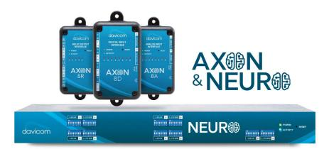
The AXON and NEURO units extend the capabilities of the Davicom CORTEX 320 system to up to 256 actions by offering modular expansion of input/output interfaces and custom logic execution. Designed for mission-critical applications, these units add flexibility, redundancy, and scale to fire station automation and alerting workflows. AXONs can also be used to remotely monitor or perform actions by communicating through IP when direct wiring to the Davicom CORTEX 320 is not possible.
